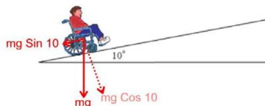
Resolving the weight of the person and wheelchair into components perpendicular and parallel to the ramp, we see that the force the person need apply to move at constant speed up the ramp is  $mg\sin 10^\circ$ . i.e.  $900\sin 10^\circ = 156 \text{ N}$ . (This is the force required to overcome the component of gravity acting down the ramp and get the chair moving with constant velocity)
